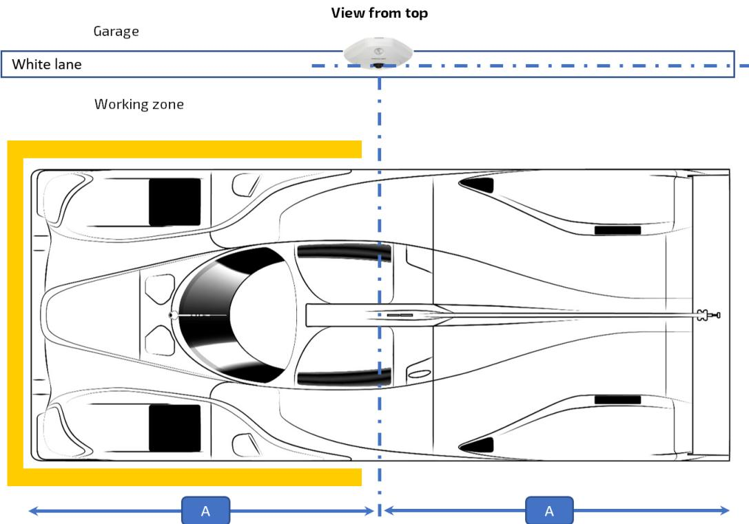
The camera must be oriented toward the car respecting an angle of  $25^\circ$  ( $+/-2^\circ$ ) from a horizontal plan:
