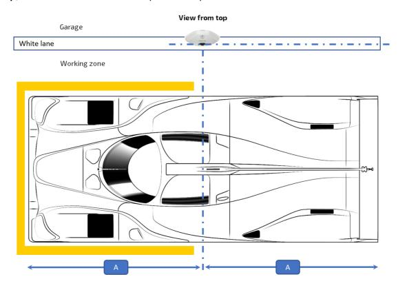
The camera must be oriented toward the car respecting an angle of 25° (+/-2°) from a horizontal plan:
