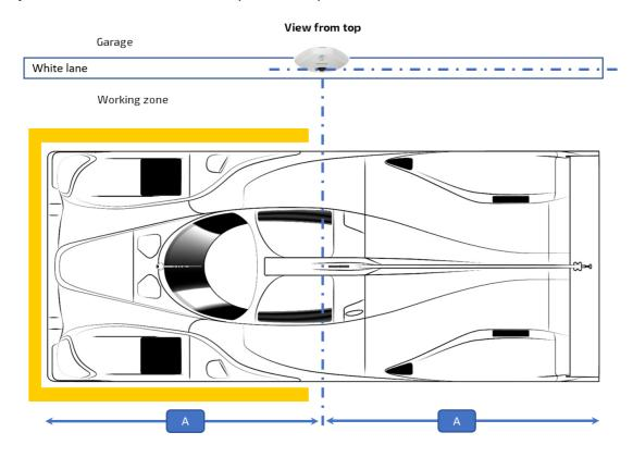
The camera must be oriented toward the car respecting an angle of 25° (+/-2°) from a horizontal plan:
