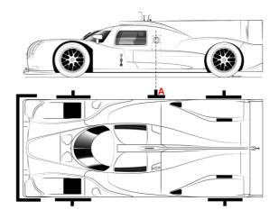
For practical reasons, the competitors shall prove FIA/ACO the difference in altitude between the described point 'A' above and the altitude of the ground at the vertical of the foremost (closest to fast-lane) point of the fuel rig (in the vertical plane, perpendicular to the pit lane line and passing through the centre of the car fuel coupling connector). This delta must be declared for each car (1 car = 1 delta) in the 'ACO TechOnline' declaration tool. (Positive when car is higher).
