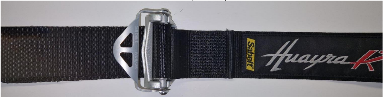
ALTERNATIVE ADJUSTER ON SHOULDER AND PELVIC STRAP (CCRE0043)
