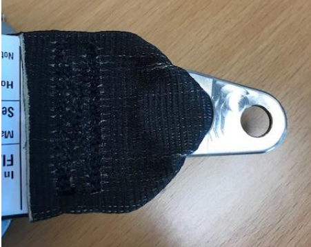
ALTERNATIVE STRUCTURAL SEAM - Near Shoulder Adjuster, Shoulder and HANS Straps Merge Point
