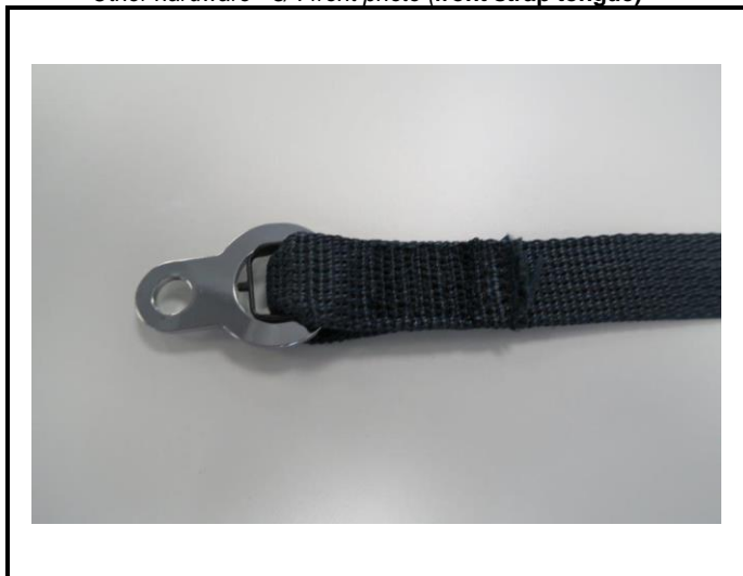
A5) Autre hardware - photo 3/4 avant Other hardware - 3/4 front photo (front strap tongue)
