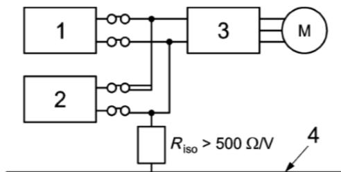
Power Ground) and Power Circuit Ground. If the monitoring system detects a DC or an AC voltage with a voltage level of more than 60 V DC or 30 V AC, at a frequency below 300 kHz the monitoring circuit must respond (within less than 50 ms) and trigger the actions to be specified in the respective vehicle Class.
