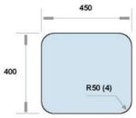
Minimum external dimensions at the section B-B
