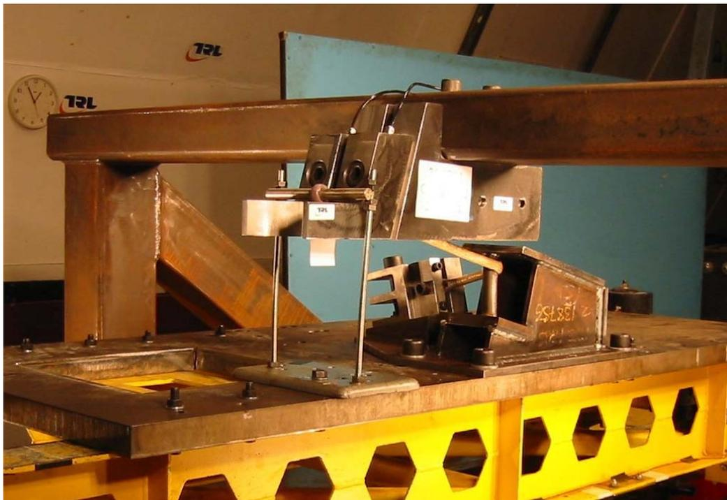
Figure A2. Test apparatus for 90° (tether sliding surface) tests on wheel restraint cables
