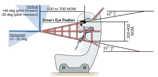
Figure 5. Positioning of net with Dual-front-attachment design
