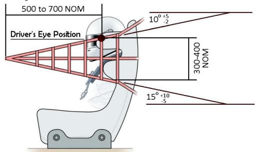
Figure 2: Positioning of net with upper-strap outside the seat-side-head
