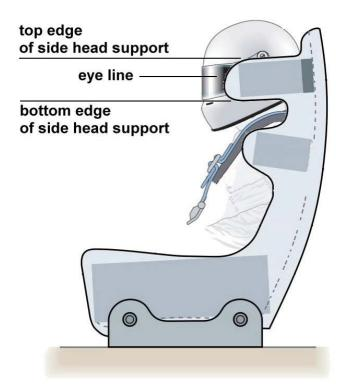
Figure A1 - Position of drivers head relative to side head support
