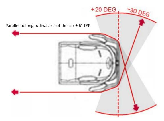
Figure 6: Attachment of front and rear straps
