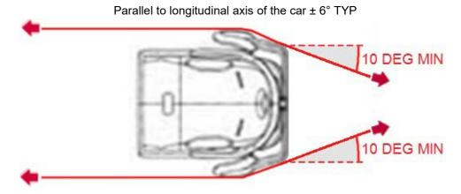
Figure 7: Attachment of front and rear straps
