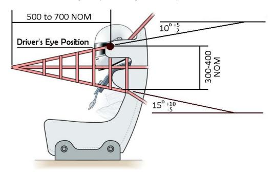
Figure 1: Positioning of net with upper-strap inside the seat-side-head
