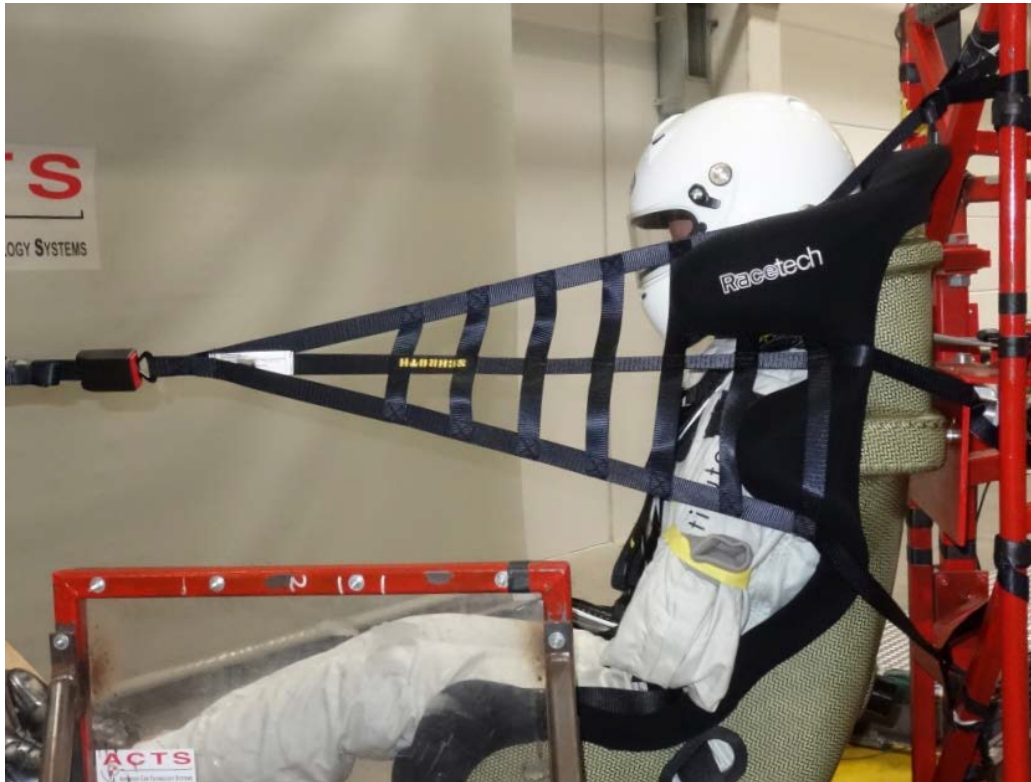
Figure 3: Photograph showing upper-strap inside the seat-side-head, shown with single-front-attachment design (external view, but valid also for Dual-front-attachment)
