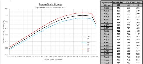
The maximum powertrain performance below 0.55 x Nmax must be lower than 246 kW.
