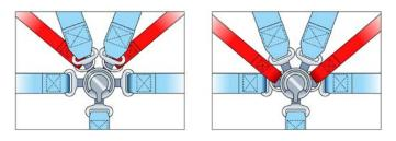
Figure 5 Examples of the SAS assembly into the seat harness buckle
