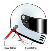
Figure 3 Identification of a Hybrid device's tethers
