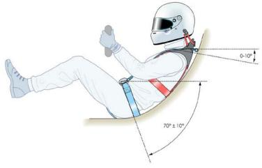
Figure 8 recommended belt angle for open cockpit cars
