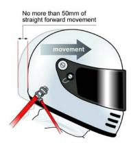
Figure 4 Movement to define the tethers adjustment
