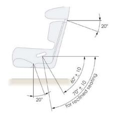
Figure 13 Side view to show recommended belt angles
