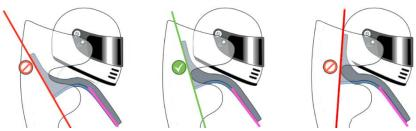
Figure 2 Examples of incorrect and correct HANS® angles
