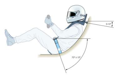
Figure 14 recommended belt angle for open cockpit cars
