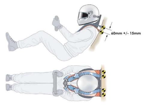
Figure 15 Installation of HANS double belts in cars where (X = < 200mm)
