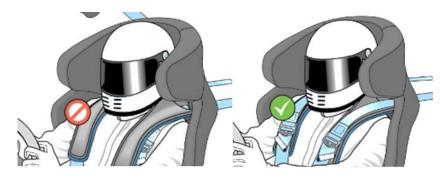
Figure 8 Example of incorrectly and correctly positioning of the harness straps when using a HANS®
