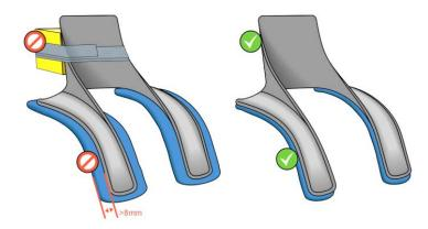
Figure 6 Examples of incorrect and correct HANS® padding
