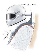
Figure 11 Minimum distance between HANS-yokes and double-shoulder belt merge point
