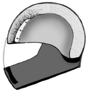
Figure 13 – Compression interne de la mousse
