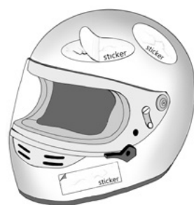
Figure 6 – Stickers covering cracks on the shell
