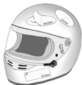
Figure 6 – Stickers covering cracks on the shell
