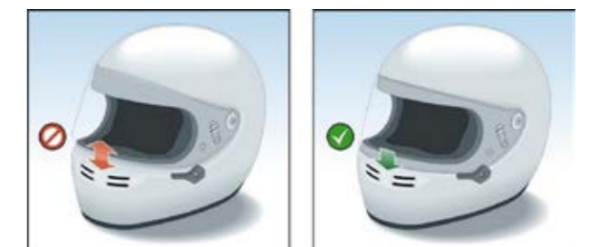
Figure 3 – Illustration of the correct closure of the visor
