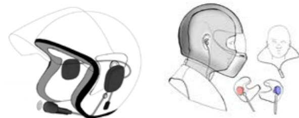
Figure 1 – Helmet-mounted radio speakers vs earplug type transducers
