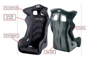
In case of cracks in the seat shell or deformation of the shell, the seat must be replaced. The crack location represents the weakest point of the seat shell. A deformed seat shell means that the seat has been subject to high loads and therefore the seat may not be able to support to the driver's body during another accident. If the seat has visible cracks, and in case of another crash, the seat may fail in that location, and may not deliver the
