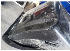
In case of damage to brackets you must check the inserts and seat shell to verify if they suffered any damage. If there is no visible damage, you may replace the seat brackets, but we strongly recommend you to contact the seat manufacturer and ask for further guidance. Please note that the bonding mechanism of the insert to the seat
