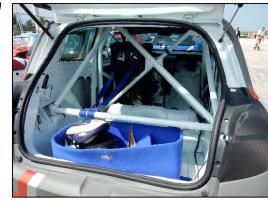
Type 2 roll cage and CS2 strut structure
