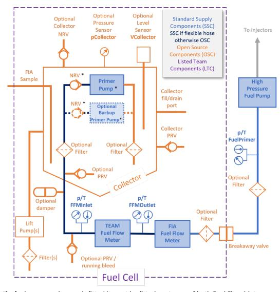
**6.6.5** If a fuel pressure damper is fitted it must be fitted upstream of both Fuel Flow Meters described in article 5.11.3.
