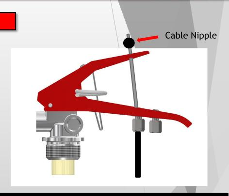
Insert the cable adjusters through the lever valve and tighten the nut.
