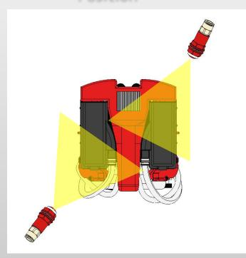
The nozzle positions play a key part in successfully bringing a fire under control and extinguishing it.
