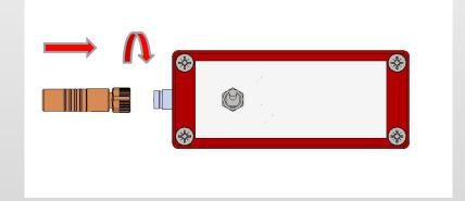
Connect one Hirschman connector to the control box using the locating slot then tighten the connector using the collar.
