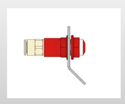
The Nozzles should always be mounted to a hard mounting point using the nut supplied.
