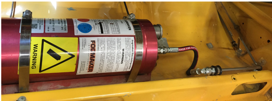
Figure 12. Connection of distribution hose to release valve
