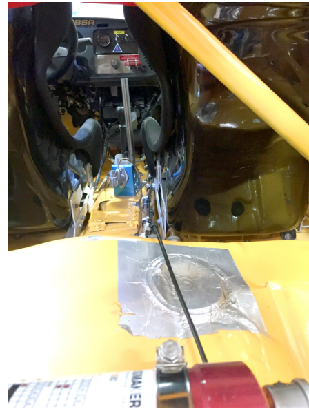
Figure 19. Installed activation handle Safety lock
