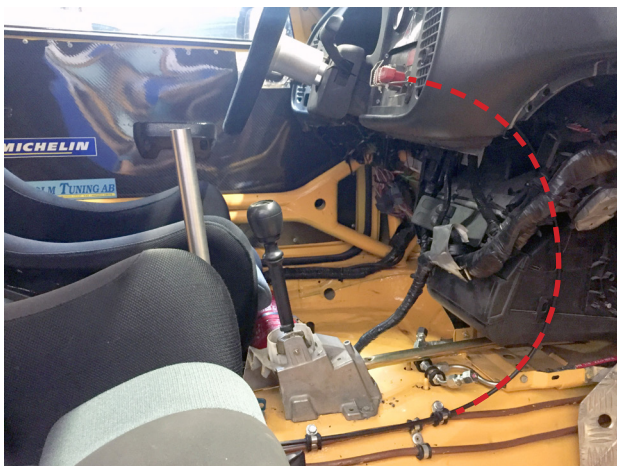
Figure 21. Wire secured with steel rubber clamps. Note the distance between clamps and the wire bending radius.
