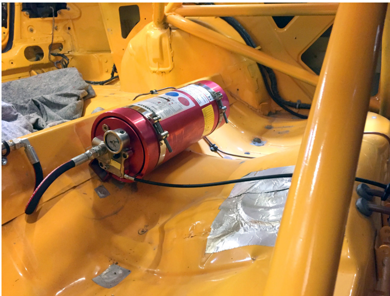
Figure 22. Ready-made wire to valve
