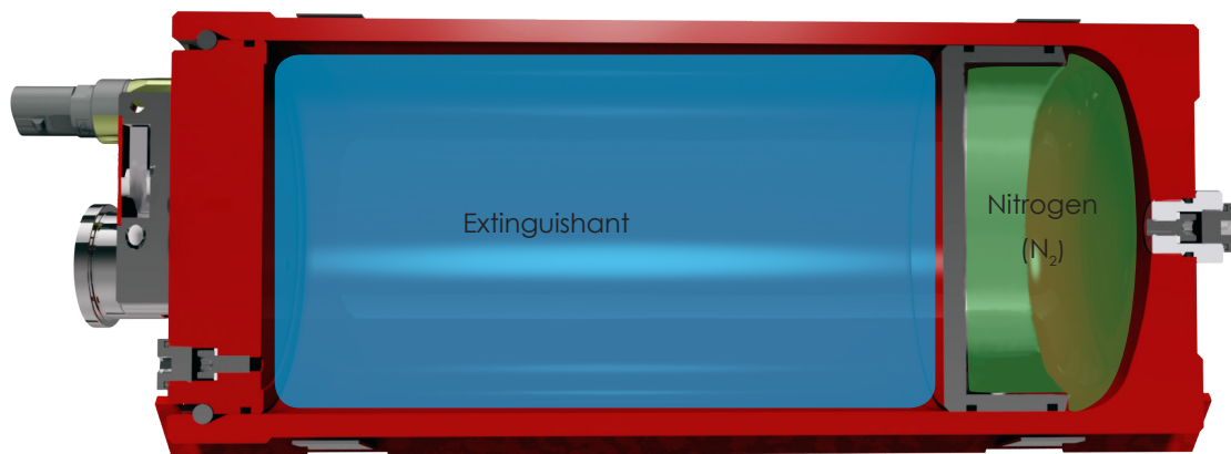
Figure 1. Cross-sectional view of a piston accumulator
