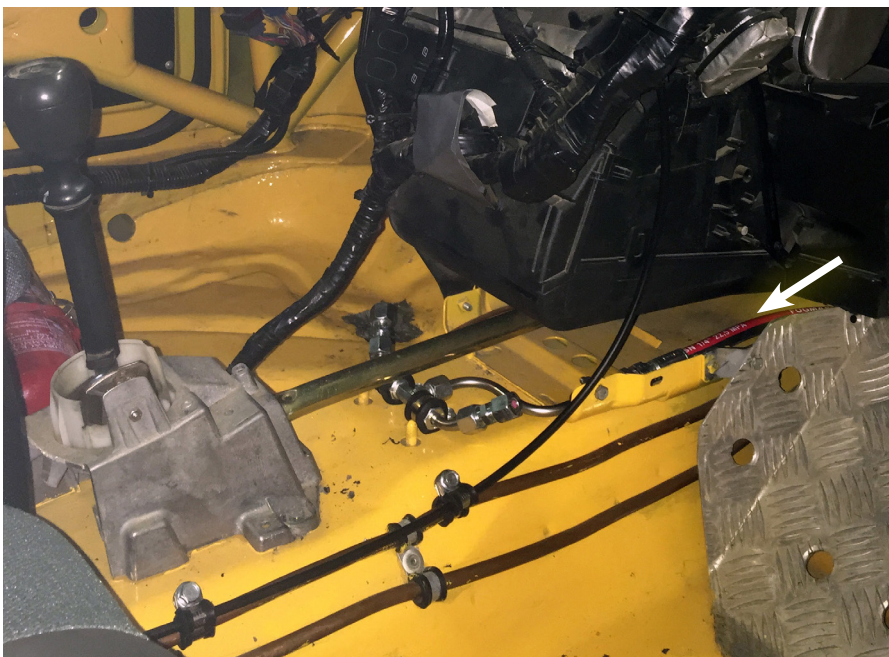
Figure 9. Distribution hose out of the engine compartment (arrow) and connected pipes with nozzles below the center console. Note that the two copper lines are fuel lines.
