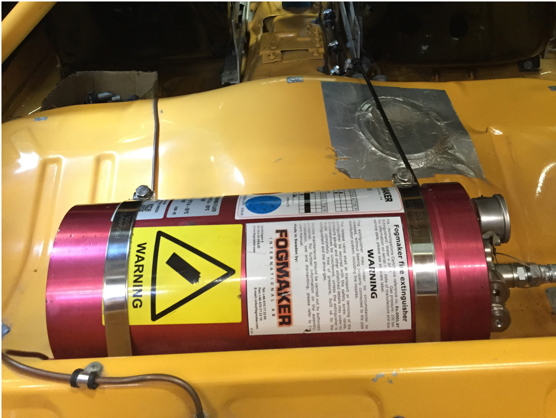
Figure 7. 3.3 liter cylinder installed in racing car
