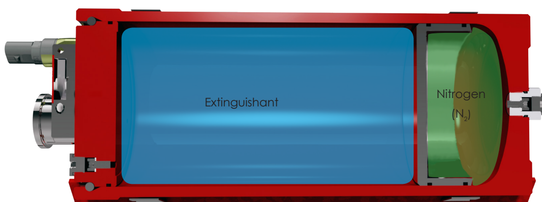
Figure 1. Cross-sectional view of a piston accumulator
