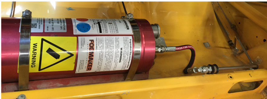
Figure 12. Connection of distribution hose to release valve
