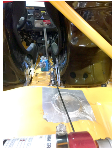
Figure 19. Installed activation handle Safety lock
