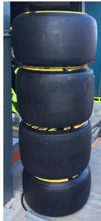
To avoid damage to the valves, it is forbidden to stack tyres as shown below:
