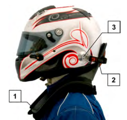
Fig. 2 The head and neck support (HANS) is a frontal head restraint device consisting of a shoulder corset (1) and two straps (2) that are fixed at the helmet (3)
