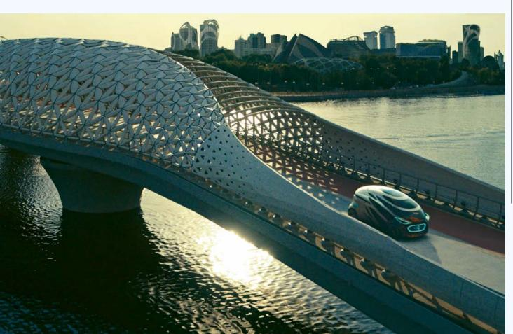
electrically-powered chassis that can utilise switchable bodies for people moving or goods transport. As a ride-sharing vehicle. Vision Urbanetic can accommodate up to 12 passengers, while the cargo module can carry up to 10 EPAL pallets. A 3.70-metre long load space fits into a total vehicle length of 5.14m.
