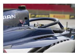
Encouragingly, the Halo on Makino's car easily withstood the ateral forces involved with being hit by another car's tyre.
