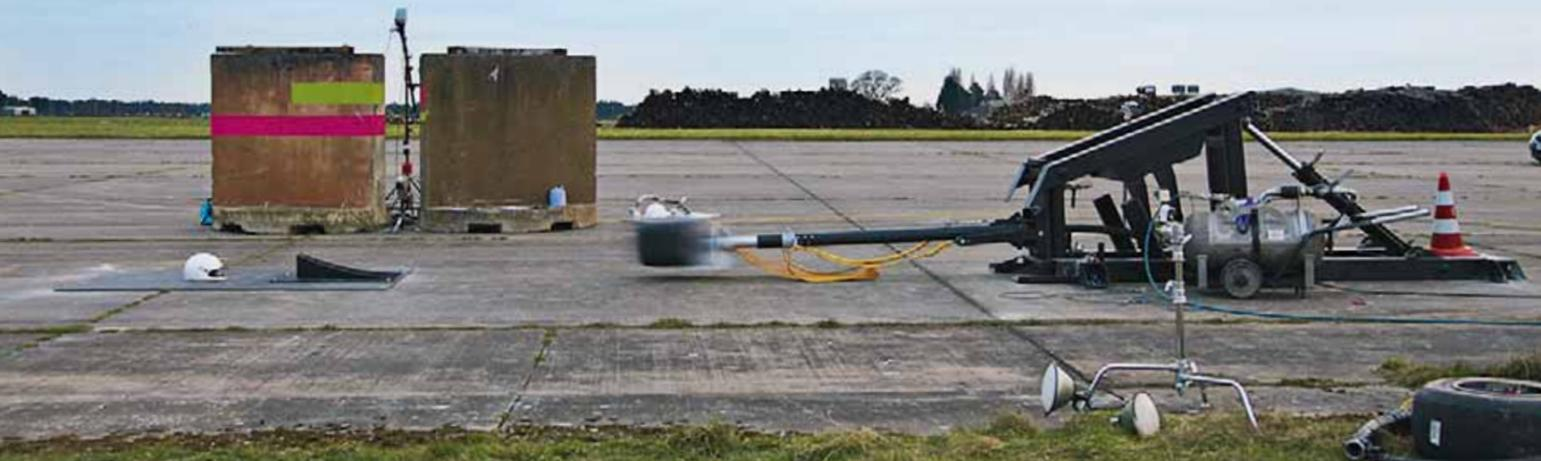
A number of tests were performed on this solution from different angles and heights and it performed well each time. The structure was extremely strong and forced the energy management into the impacting wheel and tyre, deforming the rim in all tests.
