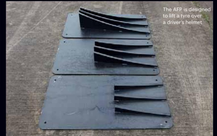
The AFP is designed to lift a tyre over a driver’s helmet
