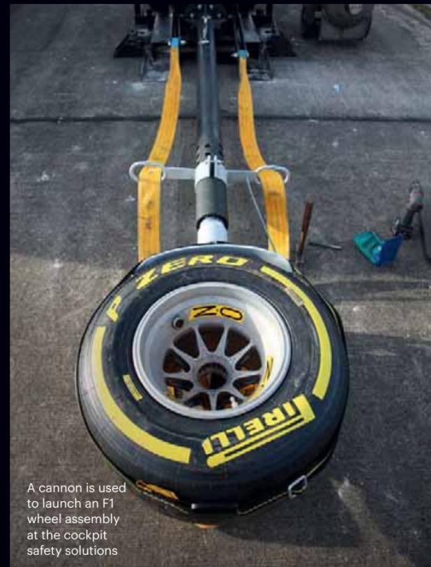
A cannon is used to launch an F1 wheel assembly at the cockpit safety solutions
