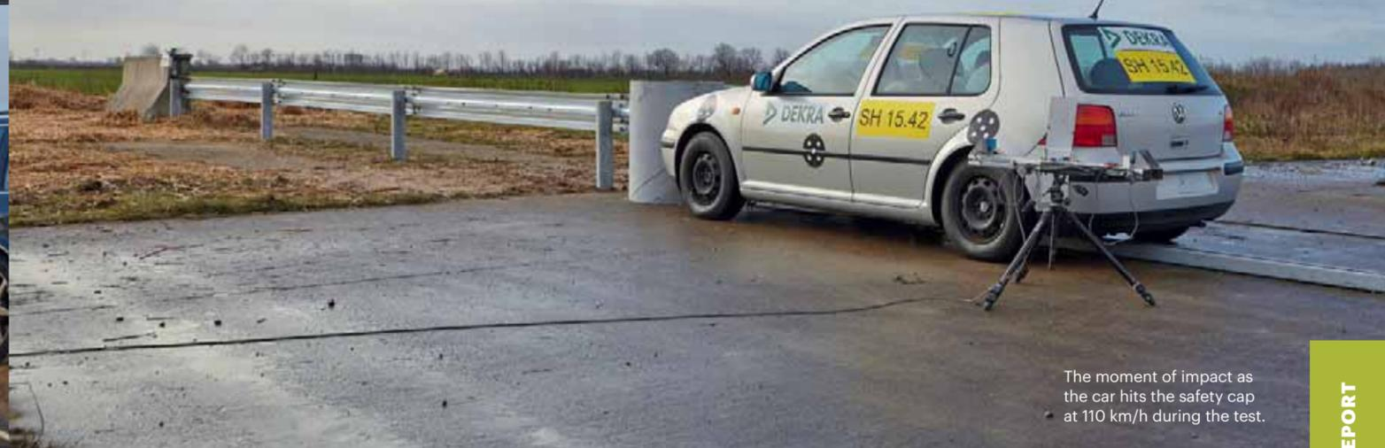
The moment of impact as the car hits the safety cap at 110 km/h during the test.
