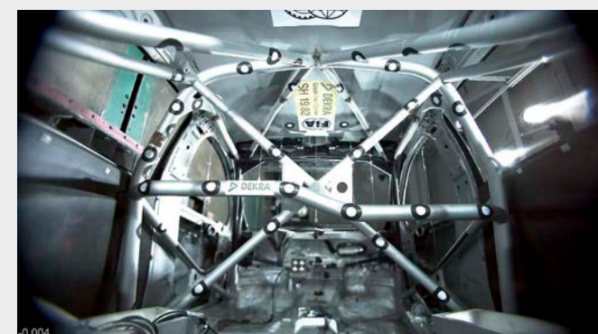
The new car will be built around a survival cell (below left) instead of the roll cage fitted into a production car.
