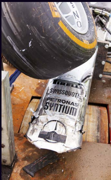
Left: the aim of the tests is to prevent nosecones from going airborne. Right: varying nosecones from four of the big teams – Ferrari, McLaren, Mercedes and Red Bull – were used in the tests.
