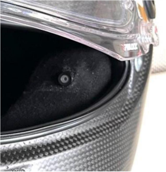
Helmet Camera - Zeronoise DE GEN 2.5 LW
