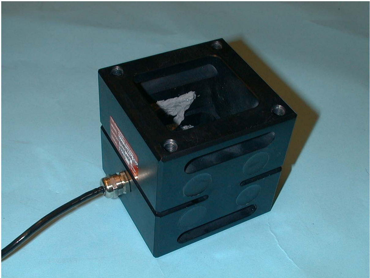
Figure C2. Photographie du capteur de force Figure C2. Photograph of the load cell
