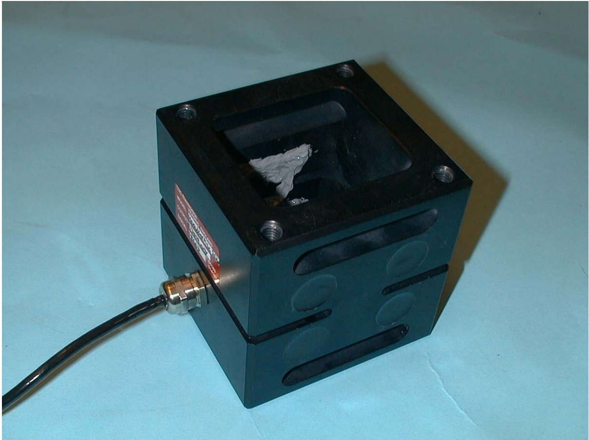
: ][ i fY&"D\ ctc[ fUd\ ]Y'Xi 'WUdhYi f'XY'Z:fWY Figure 2. Photograph of the load cell
