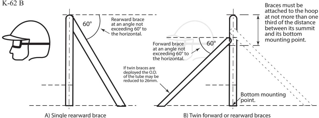
Fig 2. Roll over protection structure bracing guidelines
