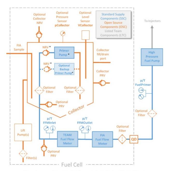
\* The primer pump(s) and the NRV(s) may also be installed outside the Collector
