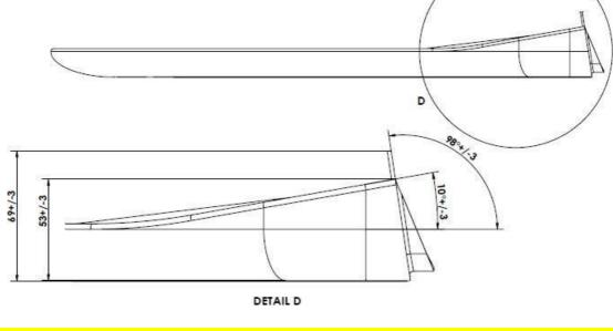
Front Splitter Brackets' design is free however the front splitter must be rigidly fixed the car's body at least in the area between the vertical projection of the front side members. Outside this area flexible front splitter mountings are allowed. (Certification)
