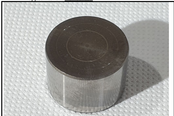
C10-6) Poussoir Admission – démonté Tappet Intake – dismounted
