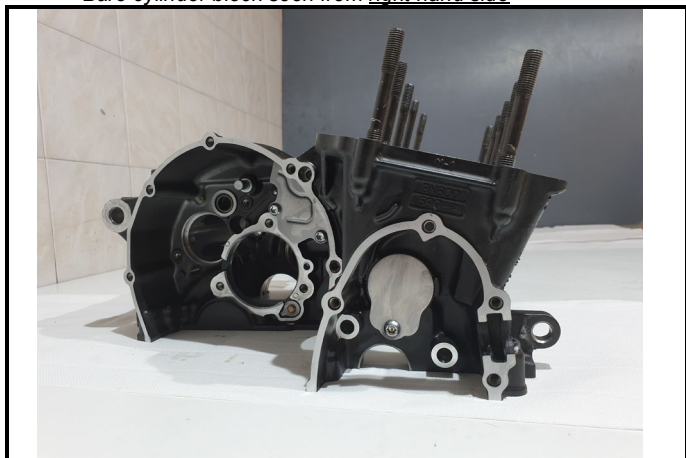
C3-5) Bloc-cylindre nu vu côté Echappement Bare cylinder block seen from exhaust side
