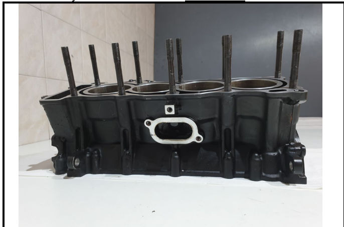
C3-5) Bloc-cylindre nu vu côté Echappement Bare cylinder block seen from exhaust side
