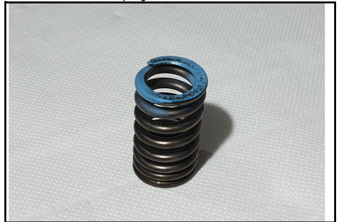
C10-9) Ressort soupape échappement Exhaust valve spring
