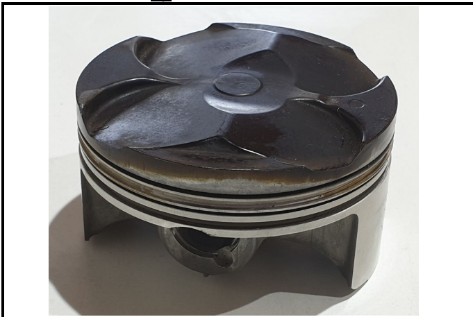
C4-3) Piston segments Piston rings
