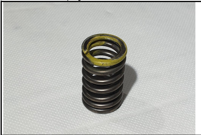
C10-8) Ressort soupape admission Intake valve spring
