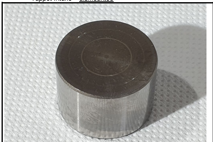
C10-6) Poussoir Admission – démonté Tappet Intake – dismounted
