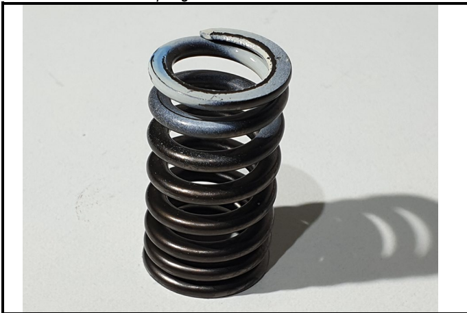
C10-8) Ressort soupape admission Intake valve spring
