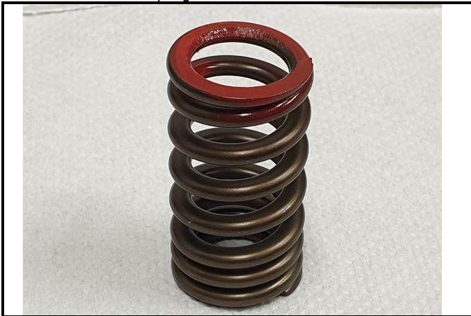
C10-8) Ressort soupape admission Intake valve spring
