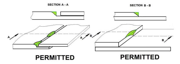
• It is not permitted to apply any kind of glue and/or filler to improve the junction in between two components. See drawing here below.
