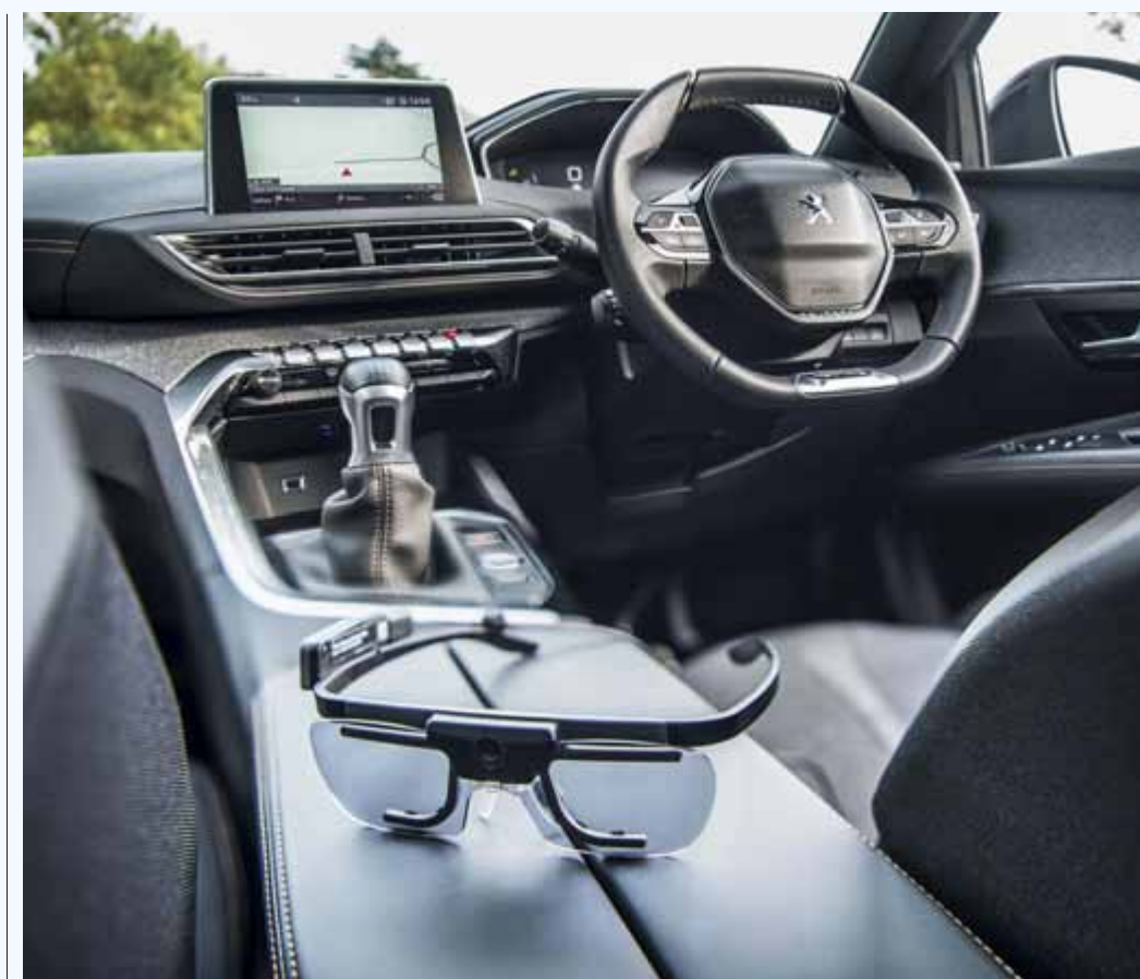
Peugeot's focus test used special glasses featuring six cameras to track the eye movements of drivers every 0.05 seconds.
