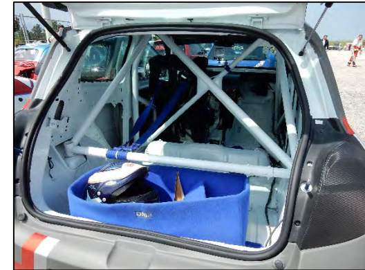
Type 2 roll cage and CS2 strut structure
