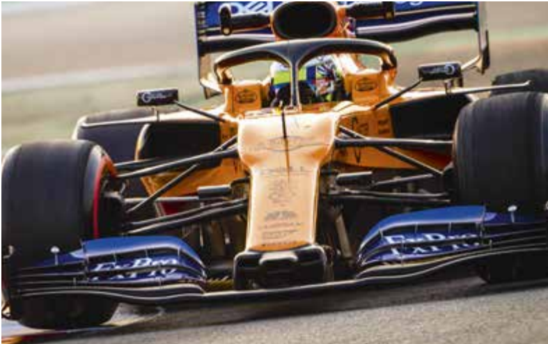
A simpler front wing, limited to five horizontal elements, has been brought in to reduce the wake effect on a following car..
