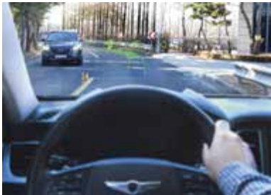
The holographic AR navigation system developed by Hyundai and WayRay AG feeds information to the driver directly via the windshield.
