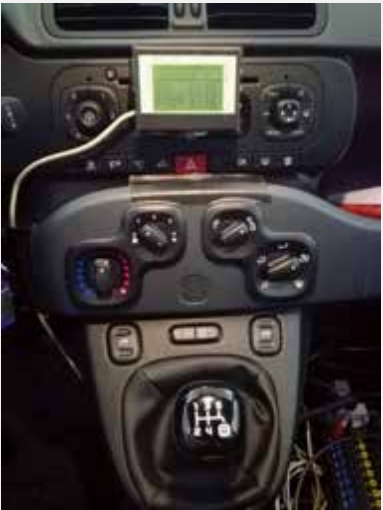
Above: The Green NCAP study featured an on-road driving test, using portable emissions measuring equipment, to accurately assess real-world emissions. Left: The FIAT Panda being assessed.
