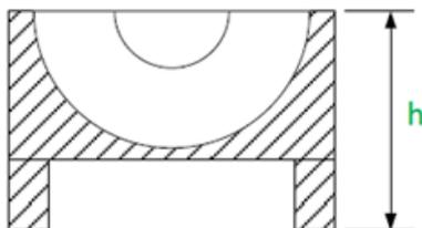
$h \geq 100\text{mm}$  must be respected for at least one cross section of the sump perpendicular to the crankshaft centreline
