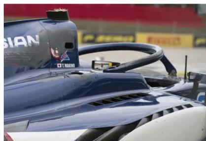
Encouragingly, the Halo on Makino's car easily withstood the lateral forces involved with being hit by another car's tyre.
