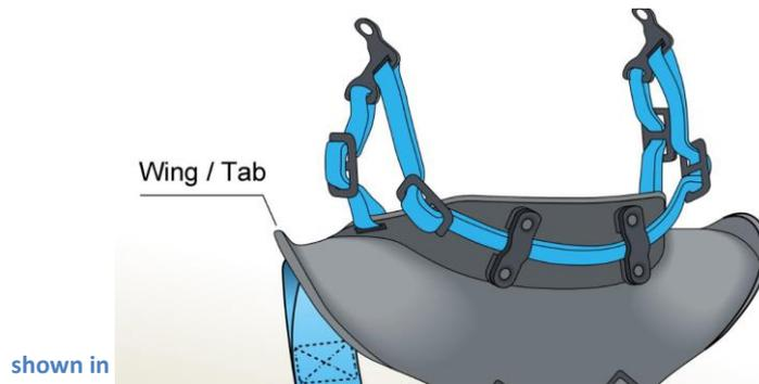
Figure 2, in order to reduce the lateral movement of the shoulder belts and retain the belts on the device.
