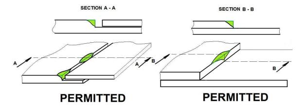
• It is not permitted to apply any kind of glue and/or filler to improve the junction in between two components. See drawing here below.
