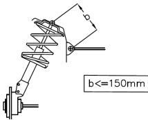
The mounting bracket may be welded or bolted to the body shell.
