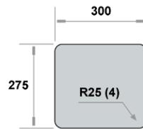
Minimum external dimensions at the section A-A
